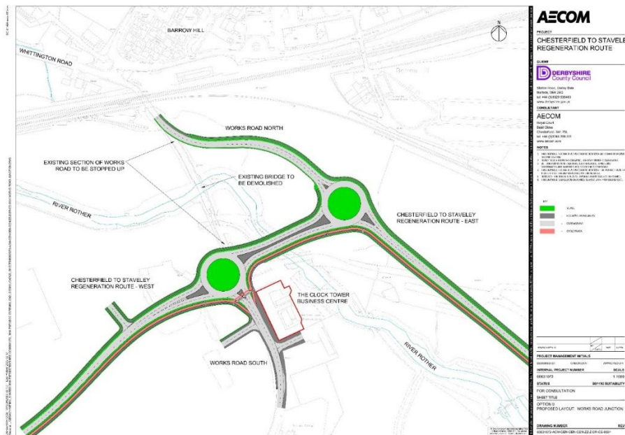
Fig 5: Detailed drawing of CSRR roundabout with spur to Barrow Hill
